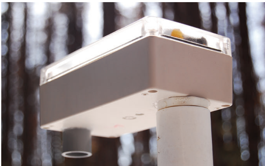
Low-cost prototype ultrasonic snow depth sensors developed for the project
