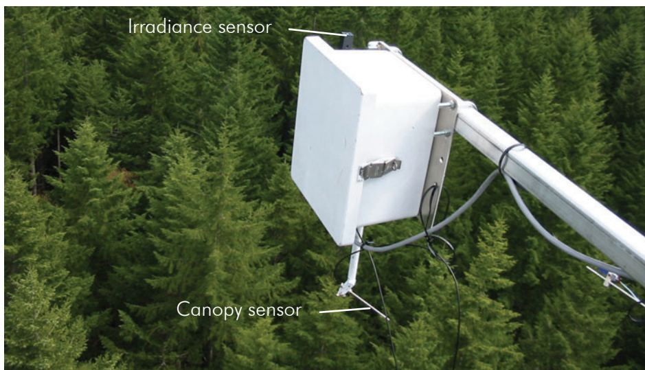
Multi-angular spectroradiometer (AMSPEC) at the research site near Campbell River, BC. The instrument is installed on a flux tower of the Canadian Carbon Program.
