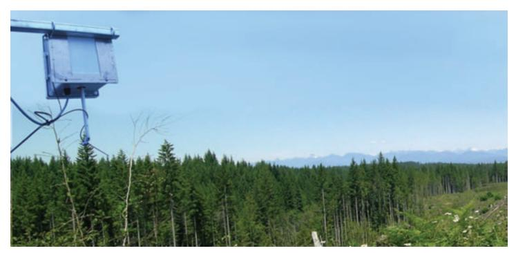
View from the top of the FLUXNET-Canada Campbell River tower with the automated spectro-radiometer measuring canopy reflectance every 15 minutes, 24 hours a day.
