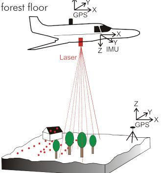
Schematic diagram showing how an airborne LiDAR system works. A laser pulse is sent from the aircraft to the ground and the beams are returned from either the ground surface or the forest canopy. Each LiDAR pulse is approximately 15 cm in diameter and is horizontally spaced at less than 1 m apart over the entire landscape.
