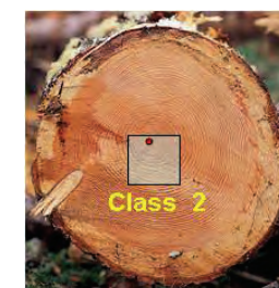
Pith location in hem-fir baby square test samples
