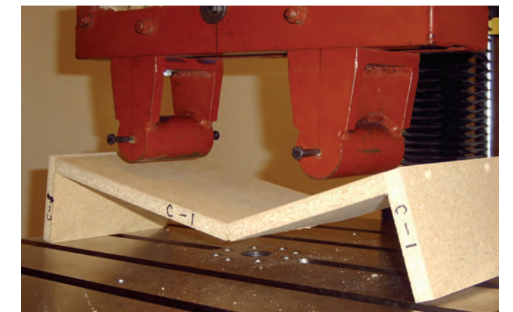
Photos show the performance of particleboard joints held together with screws: (left) failure at fastening sites and (right) joint strength exceeds bending strength of the board
