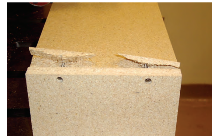
Photos show the performance of particleboard joints held together with screws: (left) failure at fastening sites and (right) joint strength exceeds bending strength of the board
