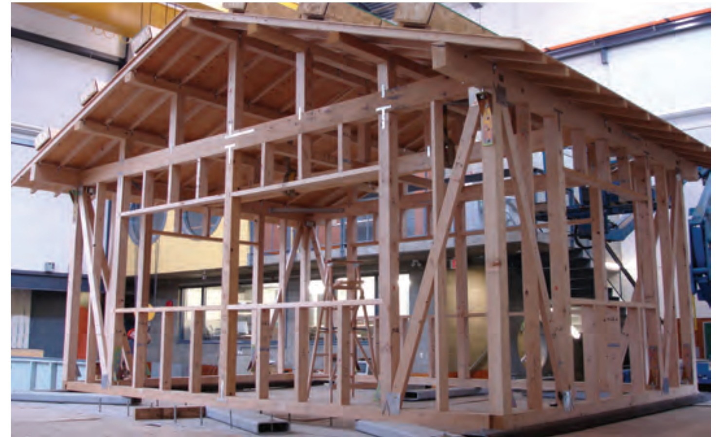
Full-sized post and beam structure at UBC's Earthquake Engineering Research Facility
