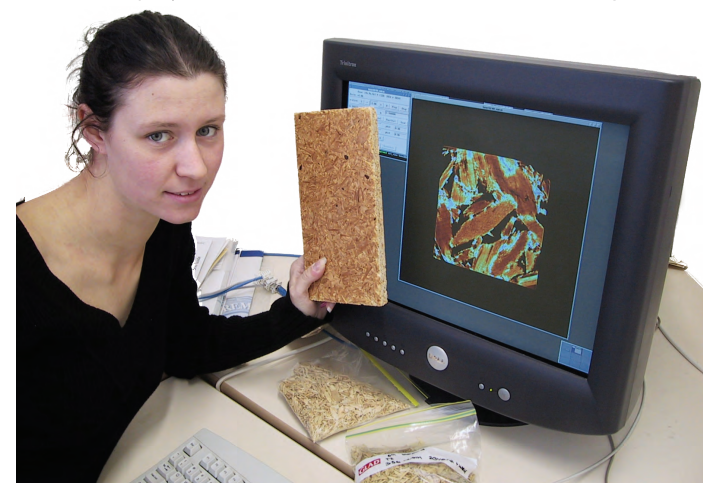
Graduate student Olivia Morrison picking out the wood from the glue using micro-computerised tomography
